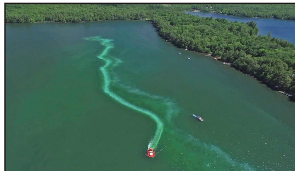
The alum trail is clearly visible behind the application barge on East Pond.
